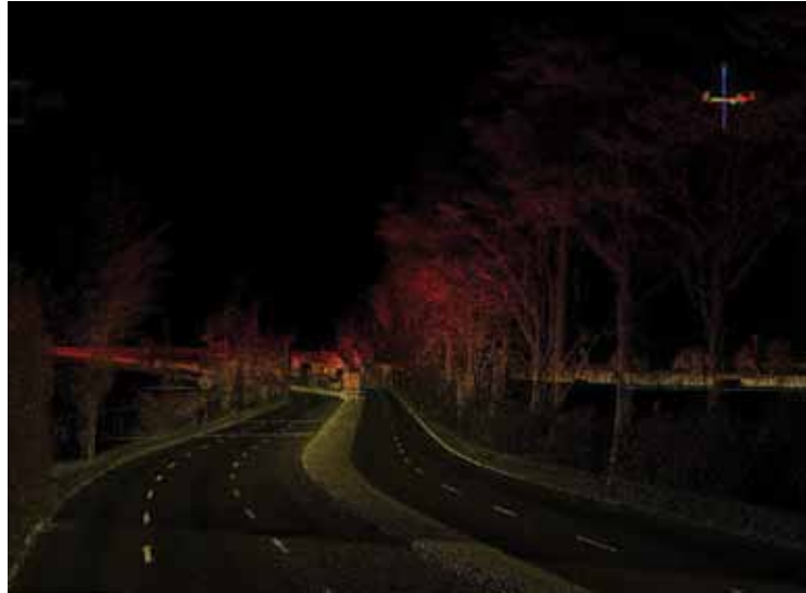
Mobile laser scanning collects hundreds of thousands of field scan points per second while traveling at traffic speeds.
