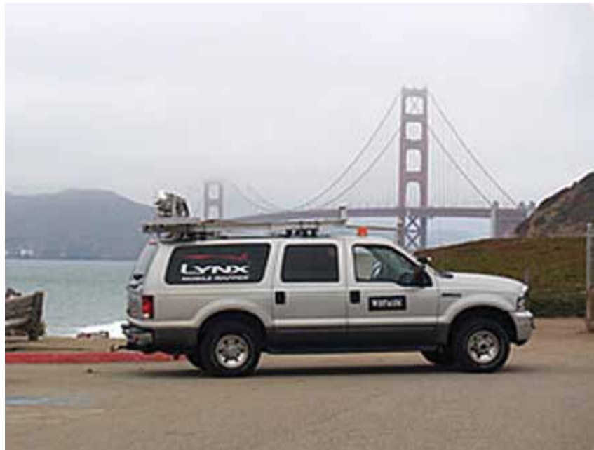
The LYNX Mobile Mapper used on the Doyle Drive project featured a tight-bundled compact Lidar laser sensor and control system with a mounting platform housing components to maintain alignment of the sensor and navigation equipment.
